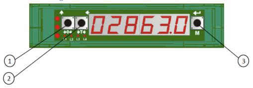
Note that the buttons have different functions for short press and long press.
