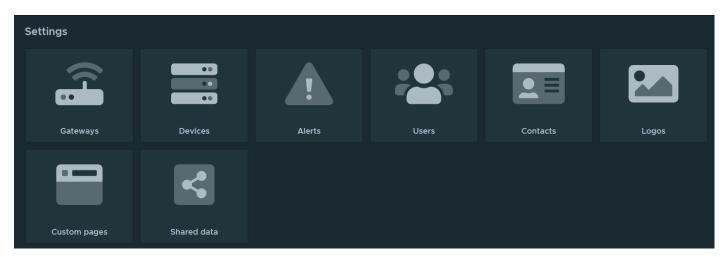
Our cloud solutions require internet access. If internet access is already available, a Data Transfer module is used for uploading the data from your PENKO instrument to the remote platform. For places where no internet access exists, a Gateway can be coupled with the PENKO instrument for uploading your data to the cloud platform.
