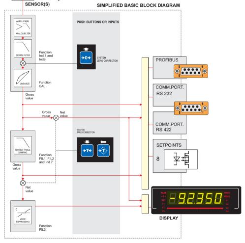
The block diagram shows the real power of the instrument. You are free to connect each value, gross, net, gross extra filtered or net extra filtered, to one of the output devices. The configuration is independent for each output. Outputs are: communication port RS232 and RS422 as well as set points. The tare system and the zero suppressing tool are connected to the display
