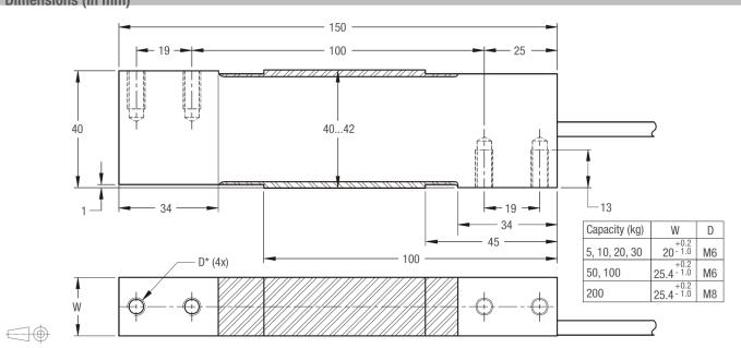
Mounting bolts up to 100 kg: M6 8.8 / torque 10 Nm; for 200 kg: M8 8.8 / torque 25 Nm. Torque values assume oiled threads. \* Unified thread 1/4-20 UNC is available.
