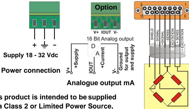
This product is intended to be supplied by a Class 2 or Limited Power Source, rate 18 - 32 Vdc, 0.4A @24Vdc.
