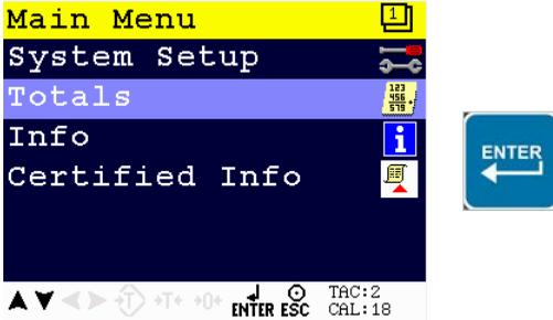
The selected totals values will be printed on the selected printer when pressed Enter.
