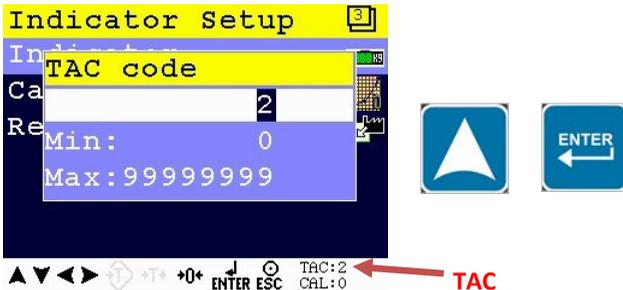
TAC (Traceable Access Code) shows on lower right of the screen.
