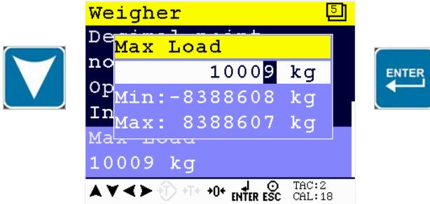
The max load prevents overload by user. Any weight above this set value will not be shown. If there is an overload, display shows the error code =====.
