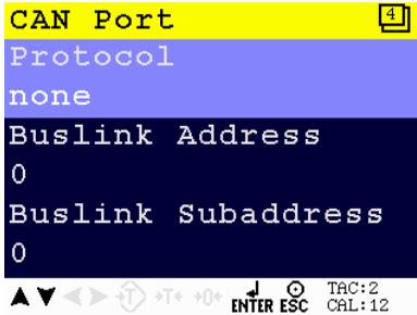
Scroll through the CAN Port menu using the UP or DOWN key. Press Enter for editing the setting.
