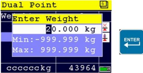
Use the UP, DOWN and LEFT key to enter the reference value. The UP and DOWN keys are used for changing the number (1-9), the LEFT key is used for changing the position of the cursor.
