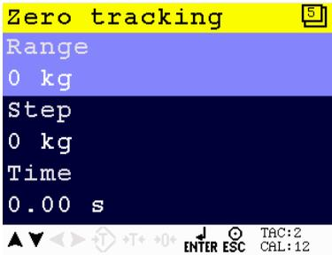
Scroll through the Zero tracking menu using the UP or DOWN key. Press Enter for editing the setting.
