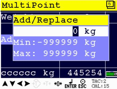
Use the UP, DOWN and LEFT key to enter the reference value. The UP and DOWN keys are used for changing the number (1-9), the LEFT key is used for changing the position of the cursor.
