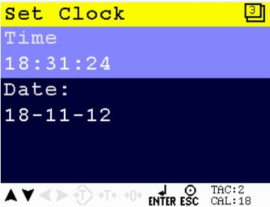
Scroll through the Set Clock menu using the UP or DOWN key. Press Enter for editing the setting.
