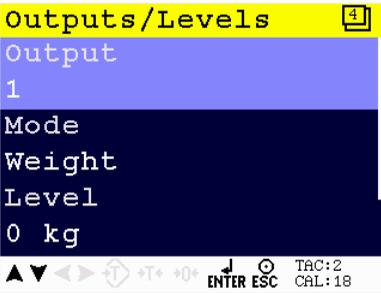
Scroll through the Outputs/Levels menu using the UP or DOWN key. Press Enter editing the setting.
