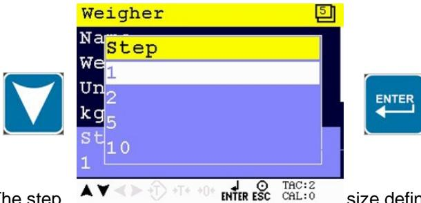
The step size defines the scaled parts of the weight value. The display value will be rounded off to the nearest value with a valid step size. Step size can be 1, 2, 5, 10, 20, 50, 100, 200.
