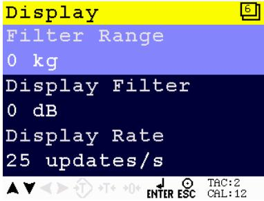
Scroll through the Filter menu using the UP or DOWN key. Press Enter for editing the setting.
