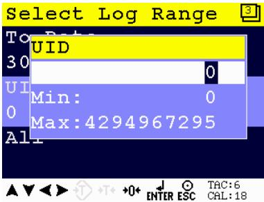
Use the UP, DOWN, LEFT and RIGHT key to enter the UID code. The UP and DOWN keys are used for changing the value, the LEFT and RIGHT key is used for changing the position of the cursor. Confirm the UID with Enter.
