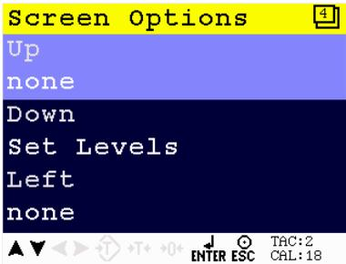
Scroll through the Screen Setup menu using the UP or DOWN key. Press Enter for editing the setting.
