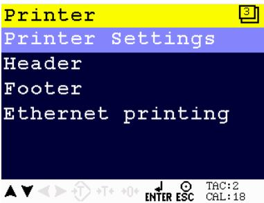
Scroll through the Printer menu using the UP or DOWN key. Press Enter for editing the setting.
