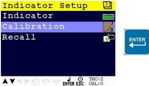
Enter **CAL (number)** by using the UP key and confirm with **Enter**.
