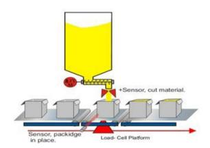
Filling of packages based on mass is applicable for solids, powders and granulates, as well as for thin and pasty liquids. Simply put, from a chemical point of view, mass is always correct. Every molecule has its own mass, so weighing means that we more or less count molecules, and is correct for all types of product.
