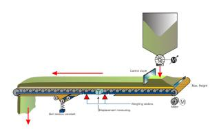
To control and regulate the continuous flow of bulk material, belt weighing systems are used. The Penko belt weighing approach detects every change in the mass flow enabling precise measurement, control and flow regulation. Penko solutions help in reducing product spillage and increasing the factory's efficiency by communication the most accurate flow.
